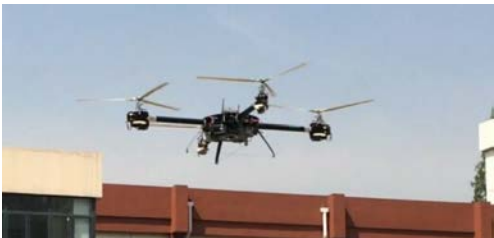
图 1 变距变转速的四旋翼无人直升机 Fig. 1 Unmanned multi-rotor aircraft with variable rotor collective pitch and rotation speed
